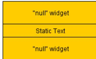
the two "null" widgets will expand equally if the frame is resized and the static text will remain centred.
