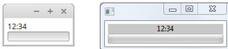
The static text in the Linux version is neither correctly aligned, nor has the correct background colour. The underlying GTK in Linux does not support text widgets with their own background panel. GTK automatically resizes the text widget to the size of the text, so even though the text is
